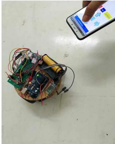
Figure 12 The photograph of smart phone and controlled car via Bluetooth communication
